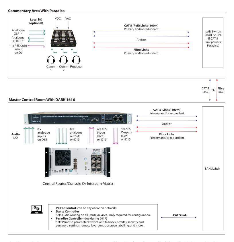
Paradiso and Dark 88 can also connect directly without the need for going through network switches. The DARK 88 and Paradiso can be set to operate in AES67 mode for compatibility with other AES67 units.
